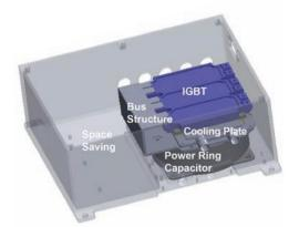
Figure 2 shows the "stacked" inverter design after the integration of the ring capacitor and the laminar bus plate. By now combining both aspects of vertical integration and the low temperature rise characteristics of the capacitors, an increase to 50% or more volume reduction is realistically possible. These improvements clearly translate into weight and cost reductions.
